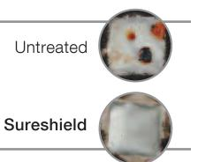
Sureshield coatings are submitted to a series of tests; before, during, and after production, to ensure superior quality. Images above give visual reference to a 28-day dried film fungal test (ASTM G 21-96). The untreated sample shows significant fungal growth and rust formation, while the Sureshield sample remains virtually unchanged.
